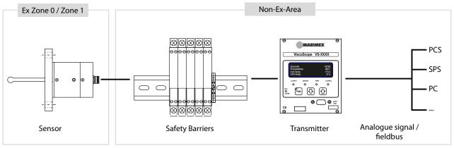
Typical system design for installation in Ex-Area
