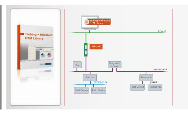
The Trebing + Himstedt DTM Library contains CommDTMs for network transition for communication with PROFIBUS DP, PA, and HART devices in PROFIBUS networks.
