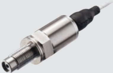
PHP160 High pressure transducer: 2000, 2500 and 3000 bar Built in electronics: 0-5V with 8-30V DC power supply High speed electronics: 5kHz bandwidth available High accuracy: up to ± 0.05% fs Compatible with on-board and test bench applications
