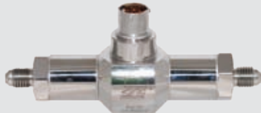
Wet/wet differential pressure transducer ±100 mbar to 250 bar uni- and bi-directional Compact with amplified output Operating temperature - 40°C to +125°C
