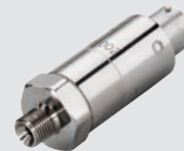
PDC220 Highest accuracy This pressure transducer includes a digital correction. Total error band up to \pm 0.1\% fs Optional temperature ranges available up to -55^{\circ}\text{C} / +150^{\circ}\text{C} Software-controlled adjustable zero and span
