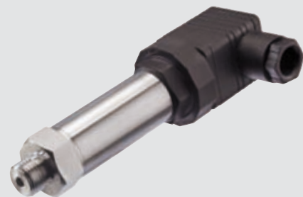
PST220 Industrial pressure transducer The high quality at a standard price Analogue outputs: mV/V, 0-5V, 0-10V & 4-20mA 1 kHz bandwidth standard
