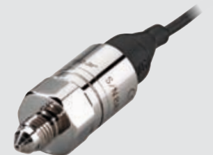
PGA220 General purpose aerospace transducer Compensated over -55^{\circ}\text{C} / +70^{\circ}\text{C} up to -55^{\circ}\text{C} / +125^{\circ}\text{C} All stainless steel, compatible with Skydrol and Kerosene High accuracy at 20^{\circ}\text{C} and in temperature
