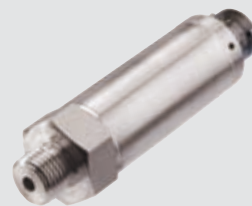
PTA220 Accurate pressure transducer High accuracy: \pm 0.1\% fs Analogue outputs: mV/V, 0-5V, 0-10V & 4-20mA Available with 0-5V - 4 wires (PTA228)
