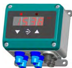
DE44 with LED-display 4 ⇒ 0...250 mbar 0/4...20 mA, 0...10 V, additional switching outputs 3-wire, M12-plug-in connector
