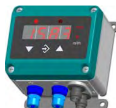
DE46 with LED-display ±12,5 Pa ⇒ 0...1000 Pa 0/4...20 mA, 0...10 V, 3-wire, M12-plug-in connector
