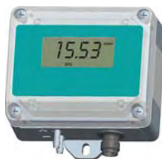
DE27 with LC-display 0...4 ⇒ 0...100 mbar 4...20 mA, 2-wire, M12-plug-in connector
