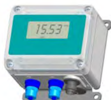
DE23 with LC-display ±12,5 Pa ⇒ 0...1000 Pa 4...20 mA, 2-wire, M12 plug-in connector
