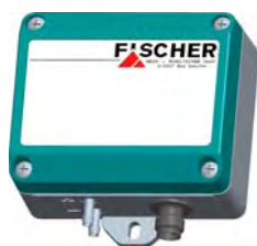
DE25 without display 0...4 ⇒ 0...100 mbar 0/4...20 mA, 0...5/10V, 3-wire, M12-plug-in connector
