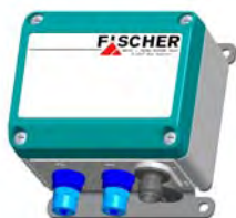
DE23 without display ±12,5 Pa ⇒ 0...1000 Pa 4...20 mA, 2-wire, M12-plug-in connector
