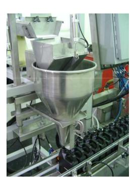
AXD load cells is perfectly adapted for high speed liquid filling
