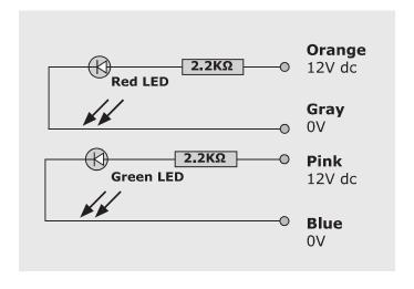
Illuminated Mullion Weatherproof Keypad with Remote Electronics
