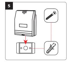
Insert the 2 plastic anchors in the holes. Place the bracket of the electronic and screw on the wall using the supplied M4x30 screws. Slide the box from up to down on the bracket.
