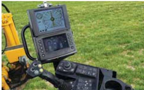
**DRILL EFFICIENTLY.** The D24x40 Series II features the DigiTrak<sup>®</sup> Aurora™ full-color touch-screen display, delivering real-time, easy-to-view locate information which can help make a driller's day more productive.
