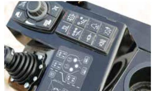
**DRILL ON.** AutoDrill allows the operator to set the rotation and thrust/pullback pressure while drilling in changing soil conditions. The Auto Resume function allows slurry/cuttings to mix before thrust/pullback resumes.
