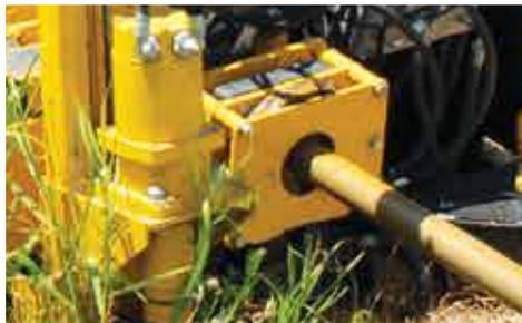
**KEEP YOUR TORQUE IN CHECK.** The torque limiter provides proper makeup torque to drill rod joints, and prevents operator from over-torquing drill rod, helping to increase life of the drive chuck and drill rod.
