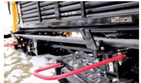
**EXTEND YOUR JOB.** Increase the length of your bore and minimize the loading time with the semiautomated add-a-rod feature. Add more rods [10' (3.1 m) rod] to maximize jobsite productivity.
