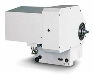
The versatile universal workhead with MT5 fitting taper is capable of both live spindle grinding and grinding between centres. The workhead spindle is mounted on roller bearings, is low-maintenance and possesses an excellent roundness accuracy of below 0.0004 mm. The fine adjustment allows for cylindrical corrections in the 1  $\mu$ m range during live spindle operations. A pneumatic lifting process facilitates movement of the workhead during setup and resetting.
