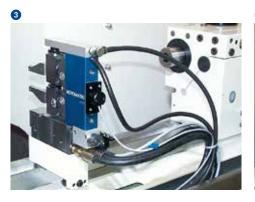
Depending on the application, different diameter measuring heads are available. They have an electric or pneumatic probe lift-off and use one or two measuring circuits, depending on the application.
