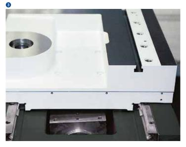
The slides rest completely on the machine base guides over the entire travel range. They benefit from the excellent straightness of the generating line, i.e. 0,0015 mm (0.000,06") over a measured length of 380 mm (14.9")!
