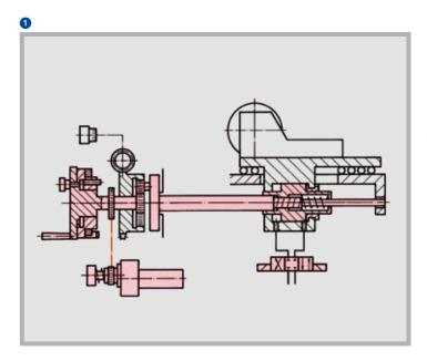
Infinitely variable feed. The cross slide is fitted with a low-maintenance hydraulic rapid approach. The pretensioned needle guides ensure stick-slip-free fine adjustment. High touching speeds and time savings are ensured by the Sensitron contact control unit (optional).
