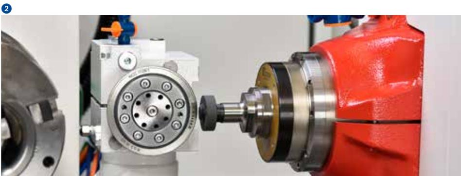
An easy-cutting grinding wheel is essential for cost-effective and high-quality grinding. Studer offers a large selection of dressing units, to allow an optimal and flexible adaption of the dressing process to the specific material, dressing tool and workpiece properties.
