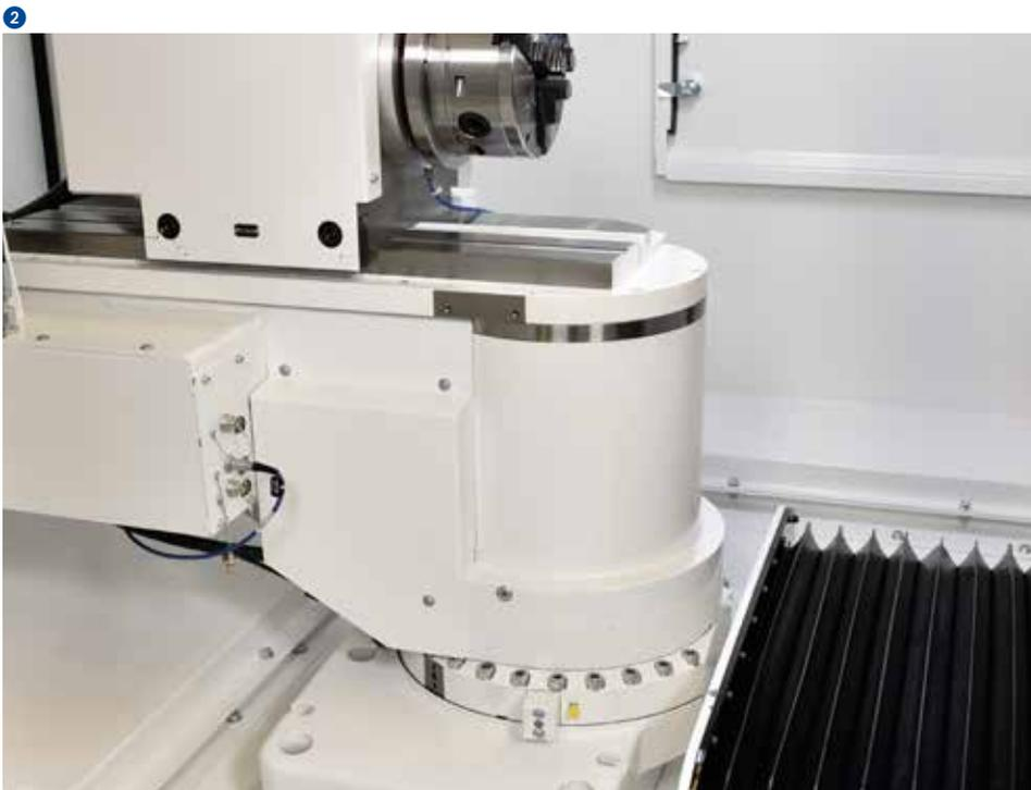
The automatic B-axis with a swiveling range of -60 to +91 deg has a direct drive, which enables very quick and precise positioning. This enables extremely precise grinding with interpolation of the B-axis to machine radii. The high-resolution direct measuring system guarantees a positioning range of the high-precision B-axis <math>< 1''</math>.
