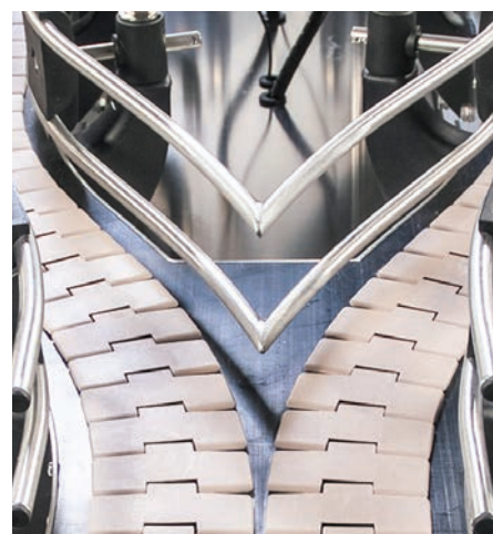
Manufacturing of customized conveyors in anodized aluminium or stainless steel with transfer curves
