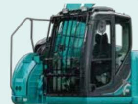
Mounting brackets for vandalism guards are standard equipment (contact your KOBELCO dealer to fit vandalism or front rock guards)
