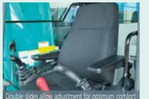
Double slides allow adjustment for optimum comfort
