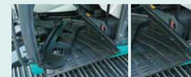
Detachable two-piece floor mat has handles for easy removal. The mat's raised edges trap dirt and grit for easy cleaning.
