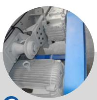
Rotor is driven via a V-belt and transmission. Equipped with a safety switch to prevent damage to rotor and transmission caused by foreign material.
