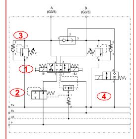
Function modules with J- or E spool could perform in On/Off operation up to zu 70 l/min and in proportional operation up to 35 l/min . The factory-provided adjustment is done via at orifice before the directional valve and /or over the spring in the pressure compensator.
