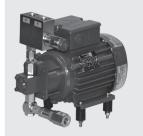
The ConditioningModule Reservoir Extraction CM-RE is designed as an accessory to the CS ContaminationSensors and the FCU FluidControl Units. The CM-RE is a self-priming motor-pump unit which makes it possible for the CS/FCU to measure oil cleanliness in unpressurised reservoirs, tanks or leakage lines.
