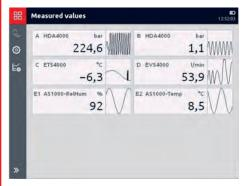
Numerous useful and easy-to-use auxiliary functions are available, e.g. zoom, tracker, differential value graph creation and individual scaling, which are particularly for use when analysing the recorded measurement curves.
