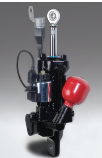
The FDE2 hydro-pneumatic semi-active cab suspension element is a combination of suspension cylinder, damping valve, and hydraulic accumulator which acts as the spring.
