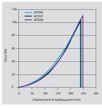
Laboratory tests by the Western Australian School of Mines (WASM) have proven that TECCO® and DELTAX® with a tensile strength of 1770 N/mm² can carry much higher static and dynamic loads than traditional reinforcement nets and are also suitable to absorb significant rockburst energies:
