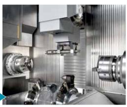
3-axis workpiece handling for flange parts
