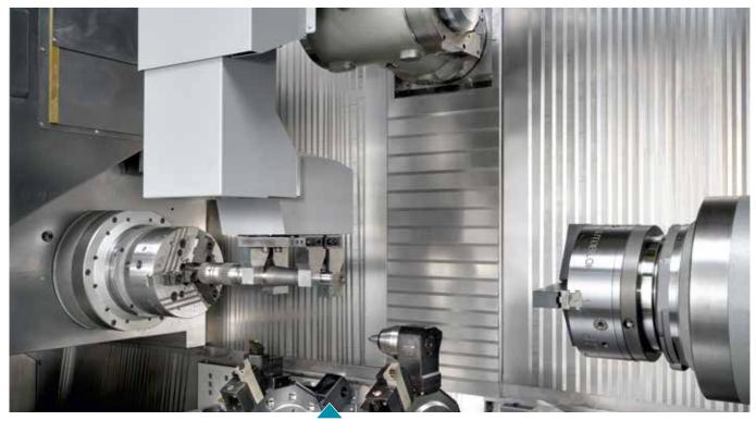
The integrated workpiece handling unit is available as an option. It can be used equally for loading and unloading as well as for the removal of remnants and is designed for parts weighing up to 25 kg and with a diameter of up to 120 mm (shaft) or 250 mm (flange). The handling unit is equipped with 2 or 3 CNC axes that are
