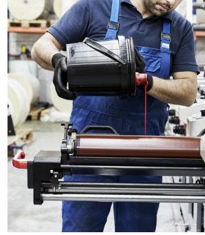
For the production of our own laminate we **Adhesive** draw from a broad spectrum that allows us to realize the right solution for your needs. Our laminate consists of three components: top material, adhesive and liner.
