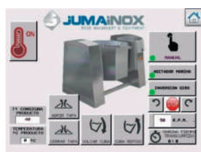
Processor with touchscreen HMI
