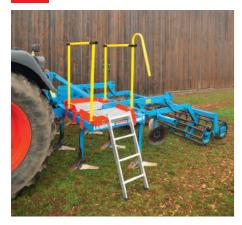
This kit allows you to safely fill the hopper. It can be added later to your soil tillage implement if there is no step or fill platform yet.
