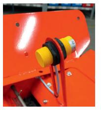
The fill level sensor triggers an alarm on the control box if there is too little seed / fertiliser in the hopper.
