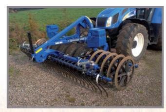
In lighter soil types, such as sand, we recommend the combination of 80cm rings on the wing sections and 11.5/80 - 15.3 wheels in the middle. Robust scrapers keep the wheels clean, and chains run between the rings allowing them to run clean.
