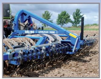
The front mounting and improved geometry actually means that the implement is being 'pulled' forwards, making it easier to steer.
