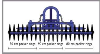
The combination of 80cm and 90cm dia rings is becoming more popular. The larger 90cm rings pack tighter the soil between the tractor wheels, whilst the 80cm rings press the soil either side. This has proven to give a better sowing capacity and more even wear on the sowing combination.
