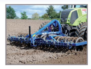
On the hydraulic folding 4m and 6m Levelflex models the hydraulic folding wing sections fold neatly to give a transport width of only 2.9m. The hydraulic folding models are fitted with an automatic mechanical locking device for transport.
