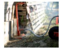
After that the cap is fixed above the hole and pressed into the ground. Now the steam can be dispersed in the pipes without pressure drop. The long and flexible gas hose between engine and slip-on cap assures a large operating range as well as comfortable working on all sides.
