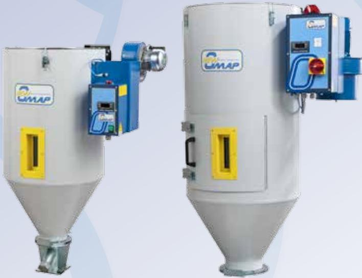
The **HD** version of hot air dryers have process airflow from 70 to 170 m<sup>3</sup>/h. These units, combined with 50 mm insulated TD drying hoppers of 15 to 200 litres volume, are suitable to be directly mounted on machine throat maximum working temperature 150°C. Supplied with their dedicated connecting base.
