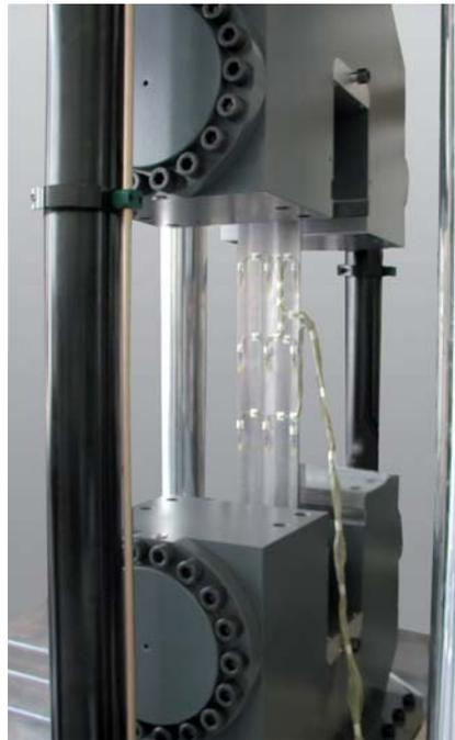
Fig. 2: Strain gaged specimen undergoing a tensile test
