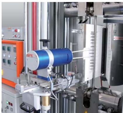
Fig. 1: High-temperature tensile test up to 1600° C
