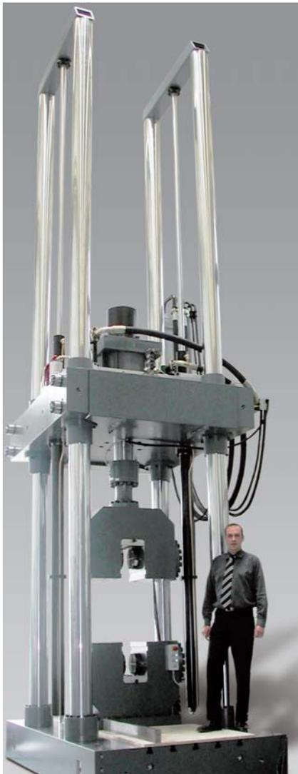
Fig. 1: High capacity fatigue testing machine HB2000
