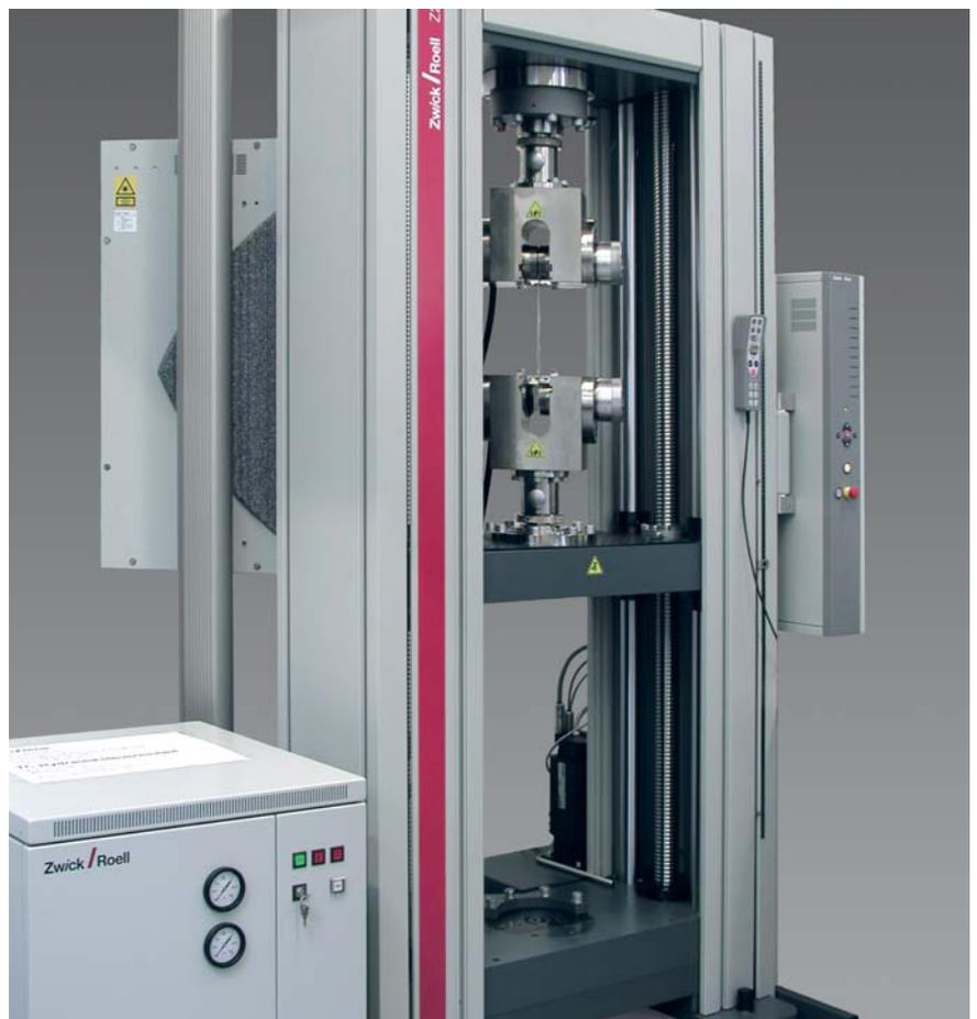
Fig. 1: Materials testing machine Allround-Line Z250
