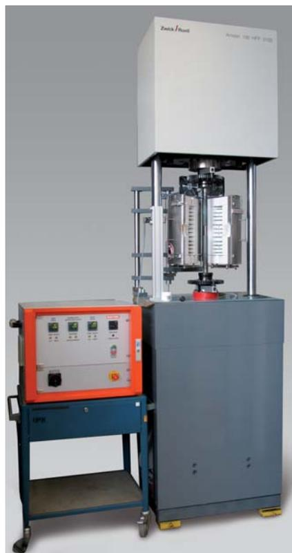
Fig. 1: Vibrophore with high-temperature furnace
