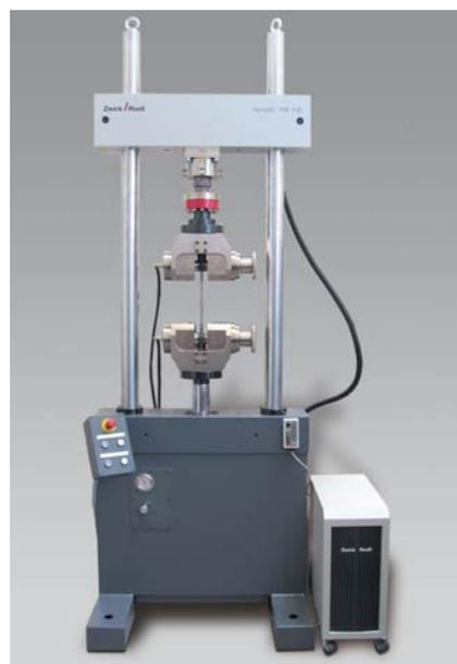
Fig. 4: Servo-hydraulic testing machine Amsler HA
