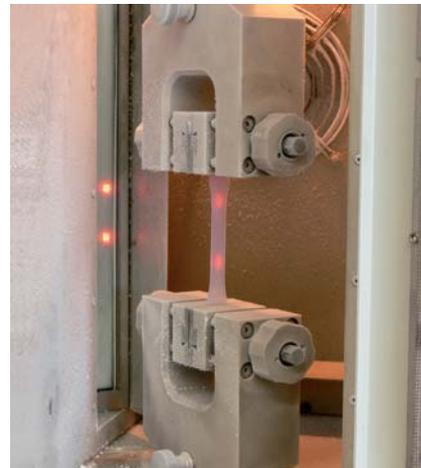
Fig. 4: Tensile test in temperature chamber up to -70 °C
