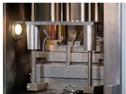
Fig. 4: Flexure test device
