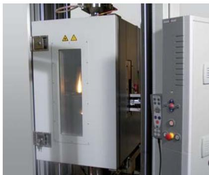
Fig. 1: Temperature chamber for composite tensile tests
