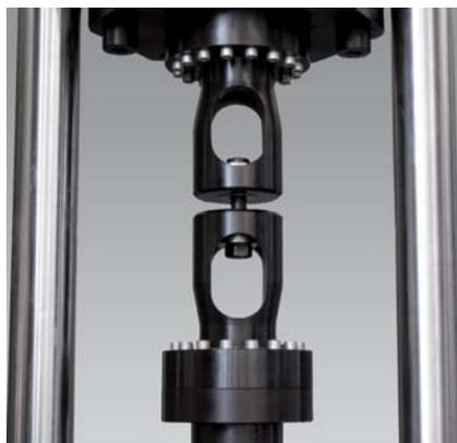
Fig. 2: Fatigue test on bolts/screws
