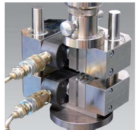
Fig. 3: Hydraulic composites compression test fixture (HCCF)
