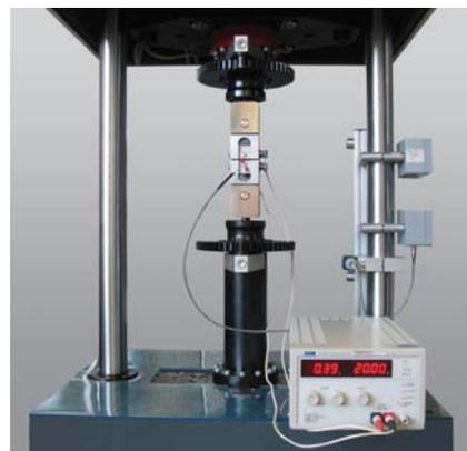
Fig. 3: CT specimen in Vibrophore (HFP)
