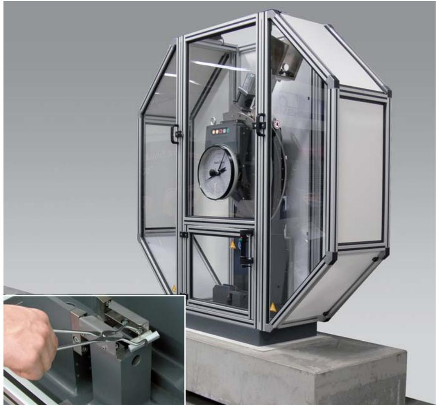
Fig. 2: RKP 450 pendulum impact tester (Inset: anvil)
