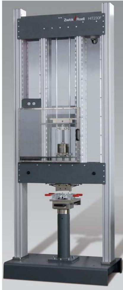
Fig. 1: Drop-weight tester HIT230F
