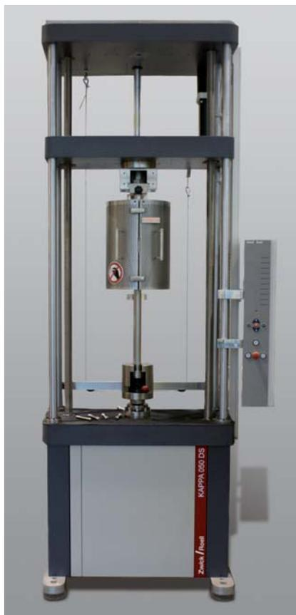
Fig. 3: Creep testing machine
