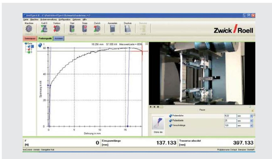
Fig. 1: *testXpert*® II with synchronized video
