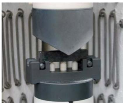
Fig. 2: High-temperature flexure test in furnace
