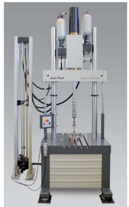
Fig. 3: High-speed testing machine Amsler HTM
