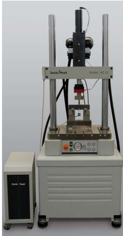
Fig. 1: Servo-hydraulic testing machine Amsler HC10
