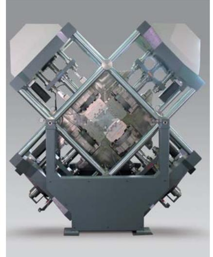
Fig. 3: Biaxial testing machine for metals
