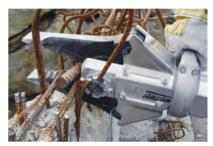
The HCS6 **C** is specially designed to expand and separate material, e.g. ripping radiators or door frames from walls or breaking up concrete pieces. The tool has a shear set for cutting-up various materials, like reinforcements up to 20 mm (0,8 inches) in diameter.
