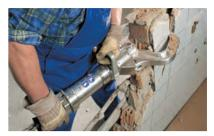
As a demolition tool, the DARDA HCS6 **B** replaces the sledge hammer as a very efficient tool that will precisely break through brick walls up to 32 cm (12,6 inches) thick.
