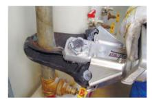
The HCS6 **S**, equipped with sickle shaped blades, is able to cut sheet metal, piping, high voltage cables, rebar (up to 16 mm/ 0,6 inches in diameter) and wooden frames. The sickle insures that the material can't slip out.
