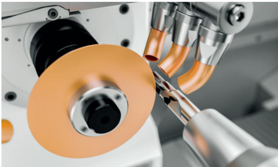
///// MACHINING A PCD STEP DRILL
