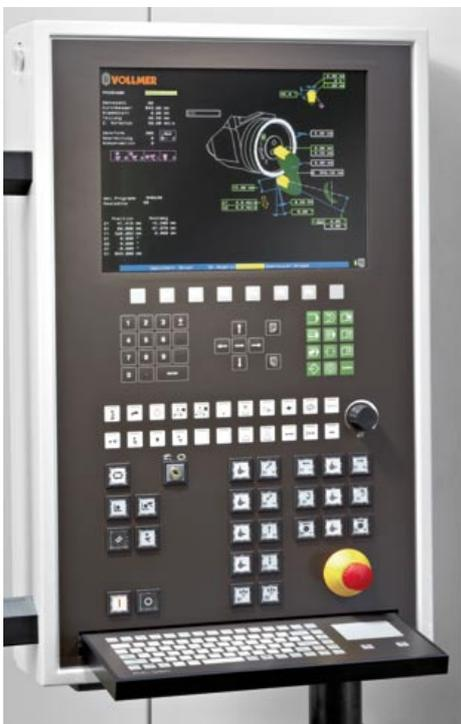
The well-known VOLLMER user interface stands for maximum operating comfort, a fast machine operator learning process, and efficient handling of the machine. A great variety of available tooth shapes offers a high level of flexibility for the production of metal cutting circular saw blades. The comfortable programming of the machine reduces also the set-up times.
