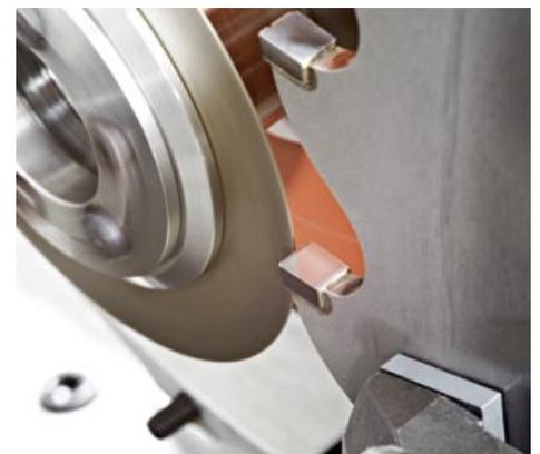
Grinding of chip breaker groove.
