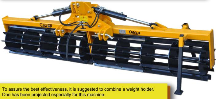
The use of rollcuts is extended to the pulverization of clods, with the condition that the soil must be dry and not sticky.
