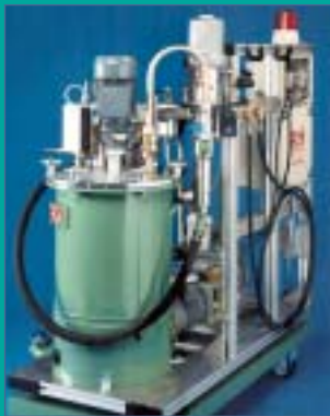
Colour dosing system for mass coloration of car steering wheels
