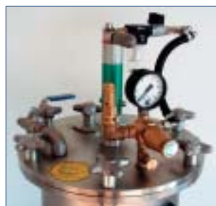
The new pneumatic agitator with a planetary gear is compact and powerful.
