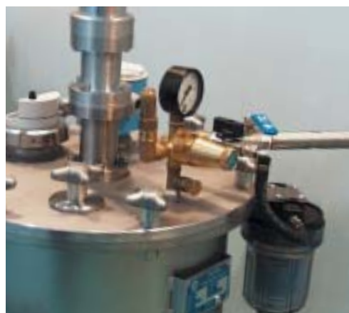
Pressure tank MDG 45 equipped with material filter and silicagel filter.
