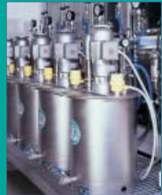
Colour mixing tanks in the automotive supply industry
