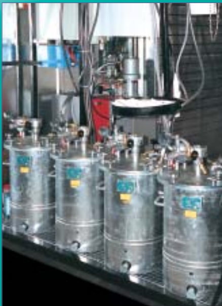
2-component system for four colours for spray application
