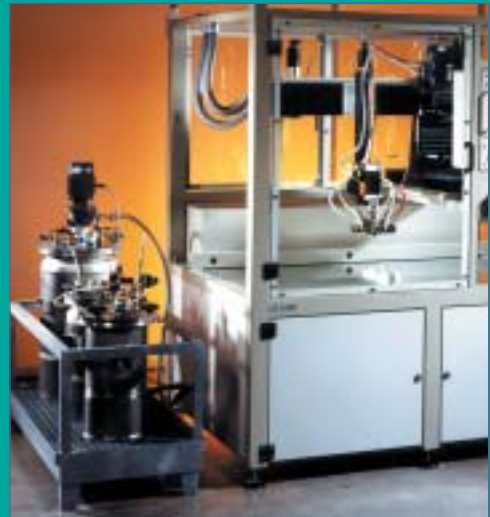
Machine for mixing and dosing two-component moulding materials such as epoxy resins, polyurethane, silicone, etc.
