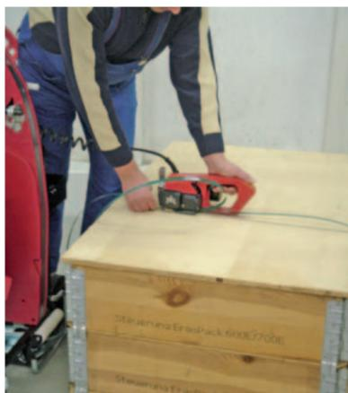
The strap will then be tensioned and sealed on the top of the pallet.
