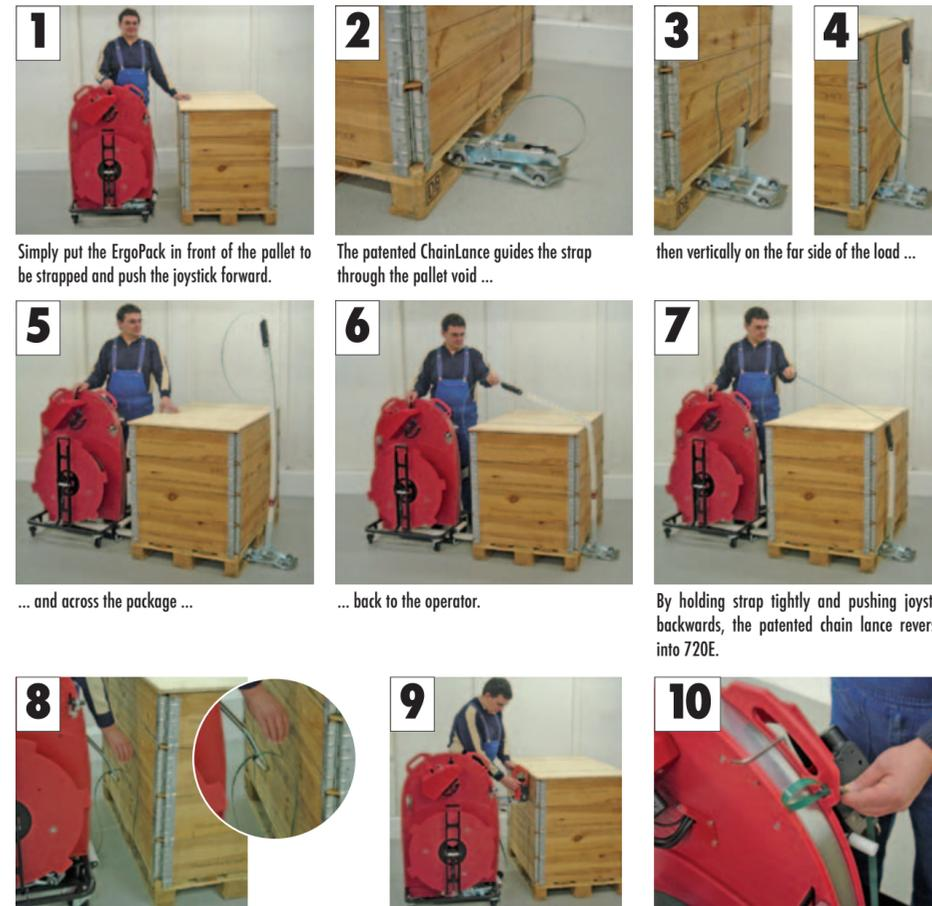
1 Simply put the ErgoPack in front of the pallet to be strapped and push the joystick forward.
