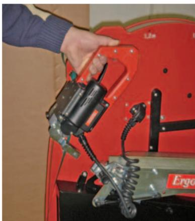
For pallets with a height below 70 cm the locking tool can be detached and placed on the package.
