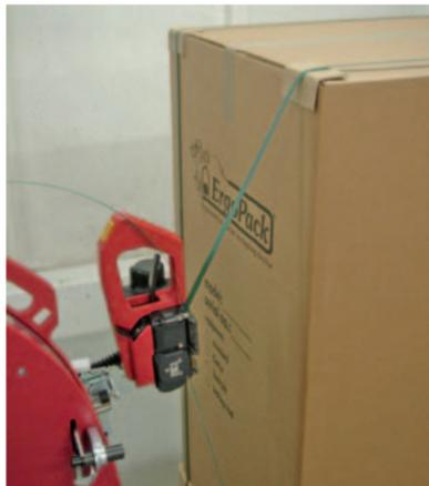
When tensioning the strap, the locking tool is automatically pulled towards the load to be packed and adjusts to its form.
