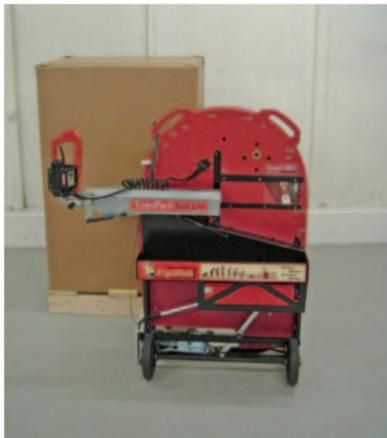
Strapping tool is supported on pneumatically operated tool lift achieving the effortless application to strap.
