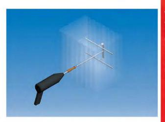
WELD-TITE MODULE Attachment is a speed weld system that requires no stud pattern or furnace layout. The advantage to this attachment system is the speed of installation. Just fire the speed weld gun which attaches the stud to the furnace casing and then fightens the module onto the stud. Nutec™ modules can be installed in a Uni-directional (with batten strips) or in a Parquet pattern.
