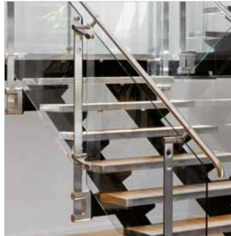
With the Blok Fixing, glass is mounted directly to the baluster post, which is then mounted to the fascia using the post's distinctive oval-shaped block. For staircases, the railing can be completed with d line Handrail. Uprights can be ordered in either 1200 or 1400 mm heights, with both intermediate and end posts available.
