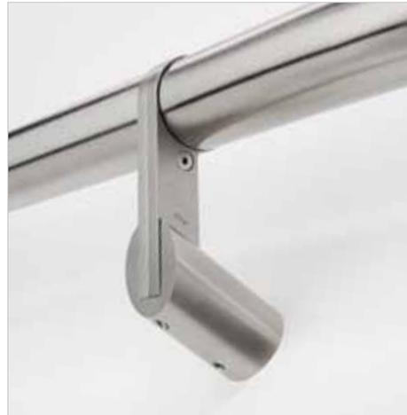
The wall rail can be installed indoors or outdoors, with or without a base rosette. The rosette fixing, which is attached to the wall using three fixing screws, is ideal for soft wall construction. The secret fixing, which installs with just one solid screw, is designed for use on concrete or hard wall construction. Both intermediate and end brackets are available.
