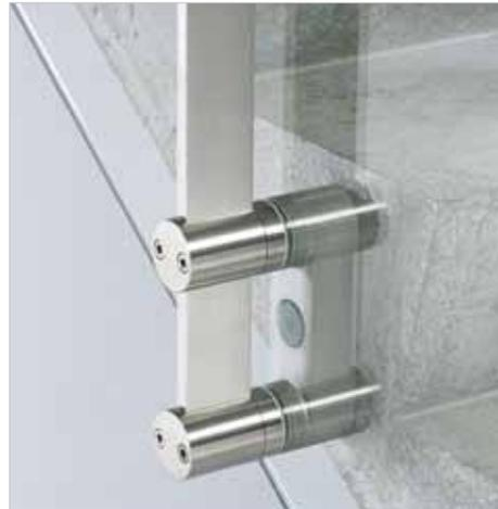
With this elegant single anchor fixed railing system the glass is mounted to the fascia with a distinctive oval-shaped block. For ease of installation, the fixing is adjustable and has level adjustments incorporated into its design. As with all d line systems, the modular components eliminate on-site welding and fabrication.
