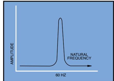
The **SPIROL** variable angle vibratory drive automatically senses the natural frequency of the feeding system and generates drive signals equal to the natural frequency to maximize the efficiency of the feeding system. It is totally independent of the main power source frequency and it compensates for changes in mass and relaxation of the springs. In practice, the drive normally operates at 25 to 35 cycles. Operation at or near the natural frequency reduces power consumption.
