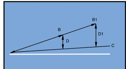
The **SPIROL** variable angle vibratory drives incorporate a system of vibration angle control. The conventional spring layout has been replaced by two separate sets of springs — one in the vertical plane and the other in the horizontal (radial) plane. The horizontal component "A" when combined with the vertical component "D" results in vibration angle "B". As can be seen in the illustration, an increase in the feed rate to "B1" does not necessarily increase the vertical component "D1".
