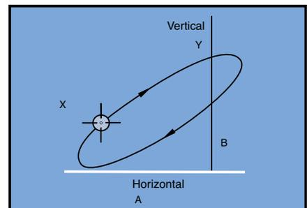
Slight adjustment of the phase control produces an elliptical motion of the bowl. The bowl does not return on its forward path but rather returns on a lower path moving away from the parts being fed. The condition is achieved where the parts are only in contact with the bowl from "X" to "Y" thus increasing the suspended motion time and feed rate. The elliptical motion also results in smoother feed characteristics as well as the separation of the parts being fed.
