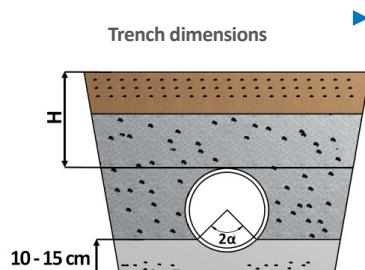
Although other types of applications are possible, **TOM® pipes are particularly recommended for underground installation**. The dimensions of the trench will depend on the loads to which pipes will be submitted (road traffic, soil types, etc). As a rule of thumb, when there is no road traffic involved, the pipes' crown will be at a minimum depth of 0.6 metres (60 cm); with road traffic, the minimum depth is 1 metre.
