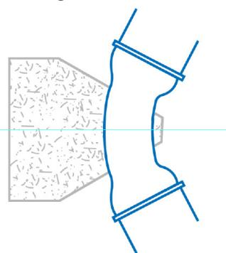
It is important to ensure that the concrete is poured directly into the previously positioned ground and that it has the required mechanical resistance. When designing the anchoring, bear in mind that **the joints must be left free** to enable its subsequent inspection during hydraulic trials.
