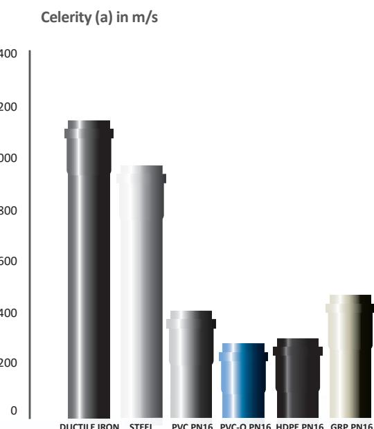
Overpressure produced by sudden pipe shut down with water flowing at 2.5 m/s.
