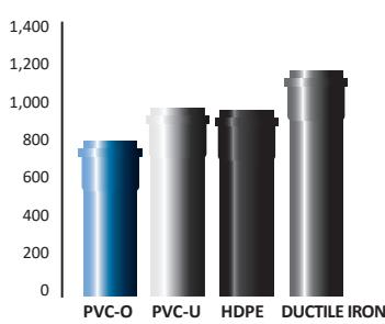
Estimated energy consumption by PVC-O, PVC-U, HDPE and Ductile Iron piping production and use.
