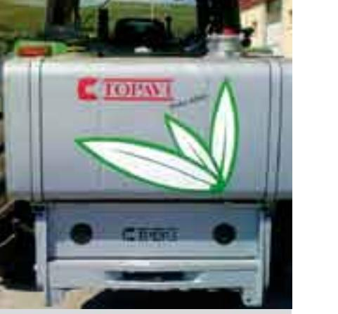
750l rear hydraulic power unit. Offsets the front-end weight of the tractor. Avoids overheating after long-term operation. With tow hook.
