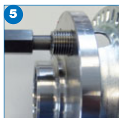
5 Checking the thread If possible, the ISO thread must be checked for trueness to gauge. The GO thread plug gauge must manually screw in to the complete thread length without application of major force. The No-GO thread plug gauge shall not manually screw into the thread any further than two rotations.
