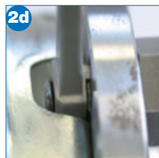
2d The cheese head screws are tightened with 50 Nm, until the punch lies flat against the thread bush. The thread bush is locked with an open-end wrench, 22 mm. After caulking, the screw joint is loosened and the thread bush screwed out.
