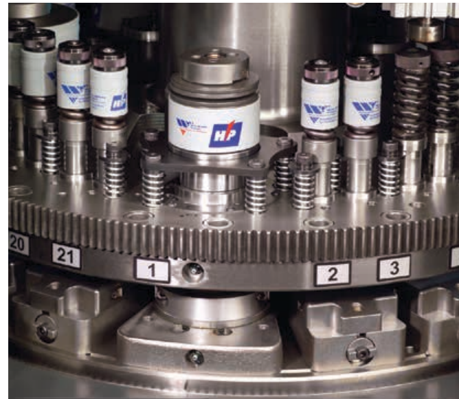
A 21-station turret configuration offers tremendous flexibility and capacity.
