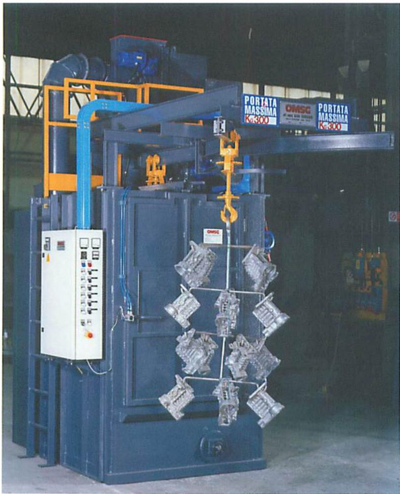
**CAPRI** Extremely versatile hook type shot blast machine incorporating a dual "Y" piece overhead handling system. Parts to be treated are hung either singularly or in batch loads onto a hook and rolling trolley assembly. Whilst one payload is inside a blasting chamber being treated, the second hook is outside the machine for off-loading and re-loading. The Capri machine is available in several models from manual loading to chains and hoists.
