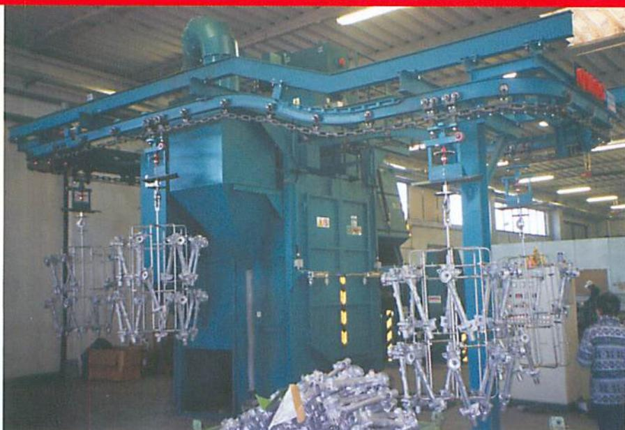
**SANDERMATIC** Tunnel type machine utilizing an overhead monorail system for conveying work-pieces to be treated through the machine. Trolleys with hooks are located at regular pitch on the ring overhead system enabling loading and off-loading on a continuous basis. The work carrying hooks revolve in front of the blast wheels giving single pass cleaning. It is ideal for mass production work-pieces and for installation on line with painting plants.
