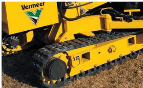
**ZERO TURNING RADIUS.** The planetary traction drive helps provide increased traction while the counter rotating tracks provide tight maneuvering in difficult jobsite conditions.
