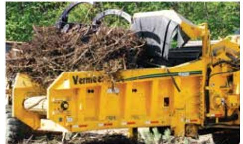
**PROGRESSIVE PROCESSING.** The patented SmartGrind system monitors engine rpm and adjusts grinding speed to increase productivity. The open-ended, wide infeed table makes material loading easy and efficient.
