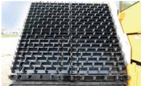
**ELEVATING FACE.** With its patented elevating-face technology, the CT1010tx lifts, inverts and aerates organic material on a single pass.
