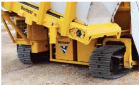
**DUAL TRACK.** Experience more control with the two-speed planetary track drive system – high for transport and normal operation, or low for wet, heavy material.
