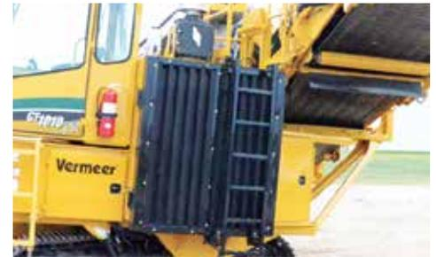
**TIER 4I ENGINE.** The Cummins 6.7 225 hp (167.8 kW) Tier 4i engine meets all U.S., Canada and European Union tier regulations, and has a 5% increase in horsepower over the previous Tier 3 engine.
