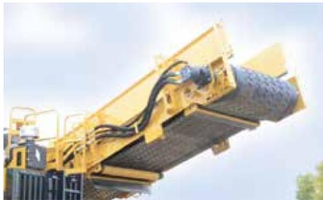
**DISCHARGE CONVEYOR.** Create a space-saving continuous stack or a 20' (6.1 m) wide by 9' (2.7 m) high windrow configuration depending on site needs and space considerations.
