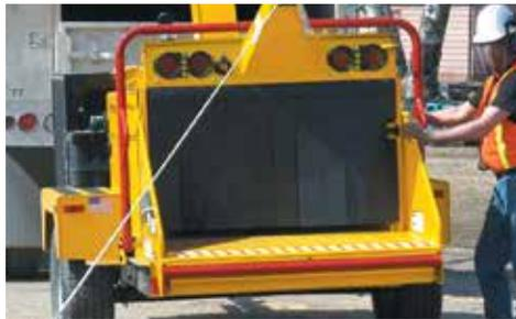
**EASILY LIFT HEAVY MATERIAL.** An optional winch allows operators to move large logs effortlessly. The 150' (45.7 m) winch line can handle logs up to 2000 lb (907.2 kg) and can automatically lift the log onto the feed table.
