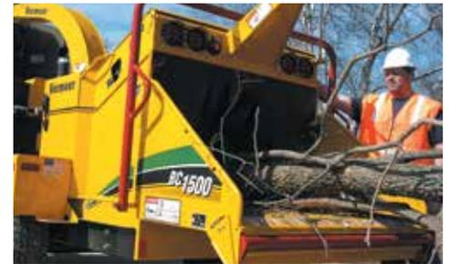
**OPERATOR SAFETY.** Mounted over the feed table, the four-position upper feed control bar enables the operator to stop the feed rollers and select forward/reverse. The patented bottom feed stop bar is strategically located to make it possible for an operator's leg to strike the bar and shut off the feed mechanism either intentionally or automatically in an emergency situation.
