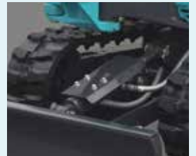
Dozer cylinder protection cover
