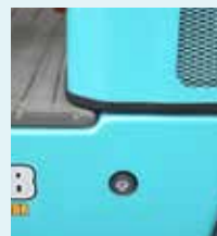
Easily checkable hydraulic oil tank gauge.
