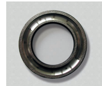
Klüberplex BEM 41-141 attained maximum run-time of 50 hours.
